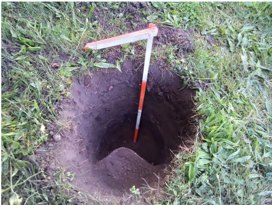
Image 20: View of disturbed test pit soil profile surrounding the farmhouse in the west of the subject property (2023). Note large rock protruding from the side of the test pit.
